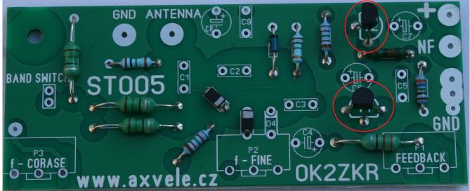
6) PCB WITH ASSEMBLED CAPACITORS C1, C2, C3, C5, C9
