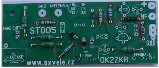
3) PCB WITH ASSEMBLED INDUCTORS L1, L2, (L3), L4
